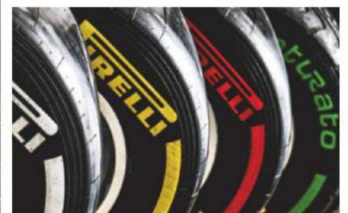
Pirelli has been the only supplier of tires to Formula 1 teams since 2011. The different color stripes on the tires signify their varying degrees of hardness, as well as their specified uses for track conditions.
